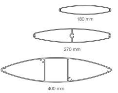
**PYLONE**'s single profiles in the shape of airplane wings range from 180 through 270 to 400 mm and have the benefit of there being no assembly required. They can be used both indoors and outdoors. The beauty of Pylone is that it can be used both for signposting as well as an advertising tool.
